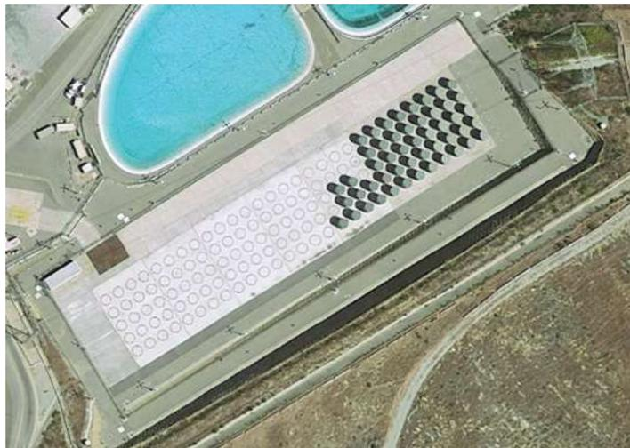
Figure 9: DCP ISFSI Pad in 2017 with 49 Loaded Casks
