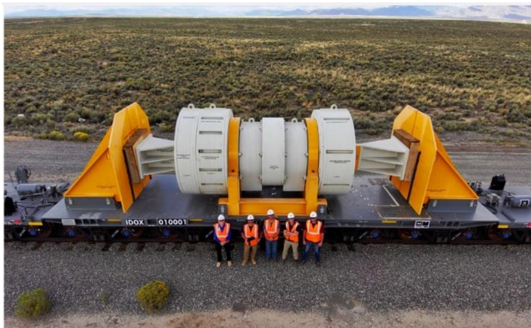
Figure 28 - Atlas railcar carrying a test load simulating a shipment of spent nuclear fuel
